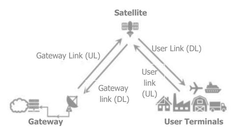
Figure 3.1: Communications links in space-based telecommunication services
