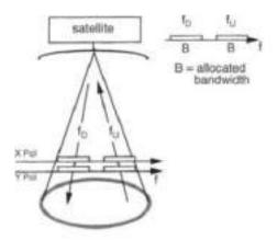
Figure: Frequency reuse using orthogonal polarization<sup>29</sup>
