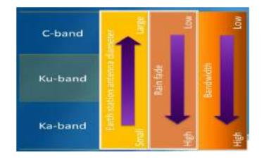
Figure 3.3: Technical Characteristics of higher spectrum bands<sup>17</sup>
