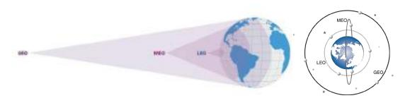
Figure 2.2: Schematic diagram of orbital altitudes and coverage areas of LEO/ MEO/ GEO satellites<sup>2</sup>
